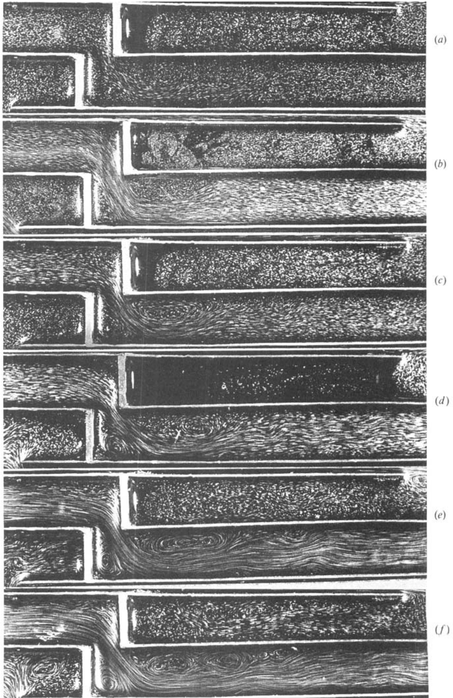
FIGURE 4. Influence of Reynolds number on flow pattern ( w/h = 0.5 ). (a) Re = 175 , (b) 300, (c) 400, (d) 600, (e) 1500, (f) 2000. Camera speed is \frac{1}{4} s for (c), (d) and (e).
